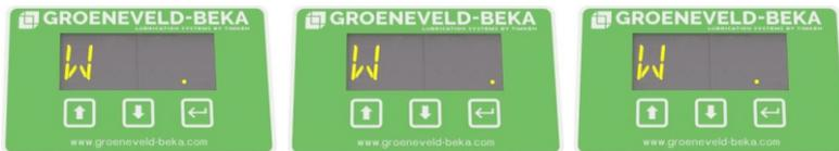
When the lubrication phase is currently active, you will see a „W“ (**Working mode**) at the first position of the 4-digit display. In the third and fourth position of the display is a dash [-] running clockwise.
