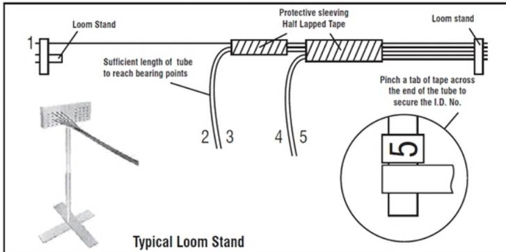
Connect the hoses to hose bundles using cable ties or tape. Protect and connect the lines using protective and spiral hoses.
